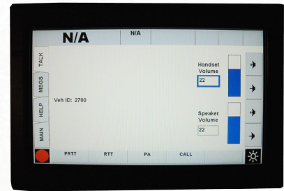
Dispatchers can send canned data messages to vehicle operators via the MDT.
